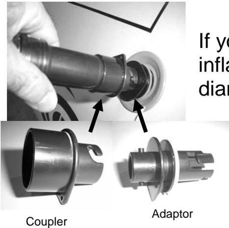
If you will be using a shop vacuum or other inflation device with a larger nozzle, use the 1- $\frac{1}{4}$ " diameter coupler (included) between the valve adaptor and the hose of your inflator. Make sure the hose is attached to the blower port of the vacuum for inflation. Insert the adapter into the air valve and lock into place by turning clockwise.
