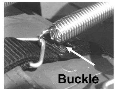
**IMPORTANT: Rotate the strap around the tube until the buckle is touching the backside of the  $\Delta$ -ring as shown.**
