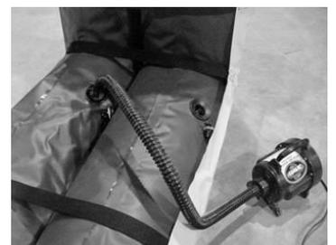
inflated. Check alignment of tubes and fit of cover periodically during inflation. If tubes are not aligned properly, release some air and move tubes to align.
