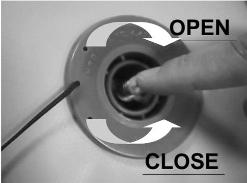
To lock open valve, depress the stem and rotate  $\frac{1}{4}$  turn clockwise. To close valve, depress the stem and rotate  $\frac{1}{4}$  turn counter-clockwise. The valve stem should be in the depressed position while inflating. Replace cap on valve after inflation to ensure air tight seal.
